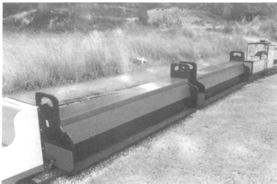
Millerbeck "Sit Astride" footboards only an inch above rail level
