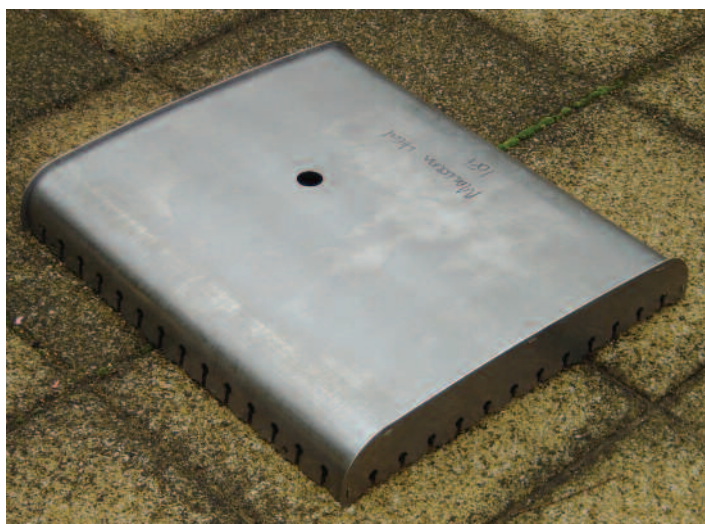
Figure 3 Canopy tabbed & slotted for welding
